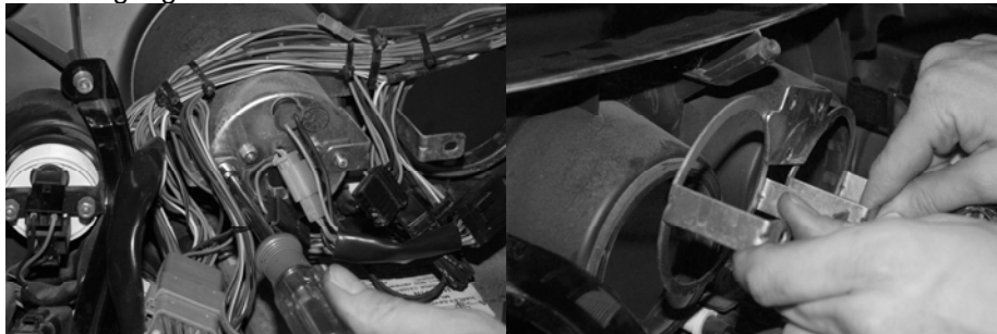
Remove nuts/screws and clamp to remove factory gauges
